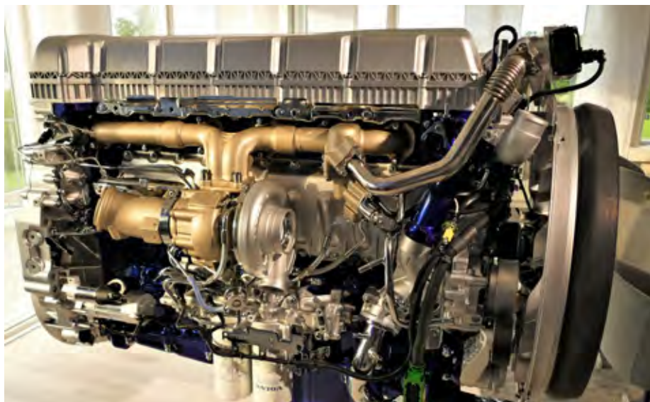
Motor, kakršen poganja ta tovornjaka, ima turbokompresor, nima pa sistema Turbo compound.
